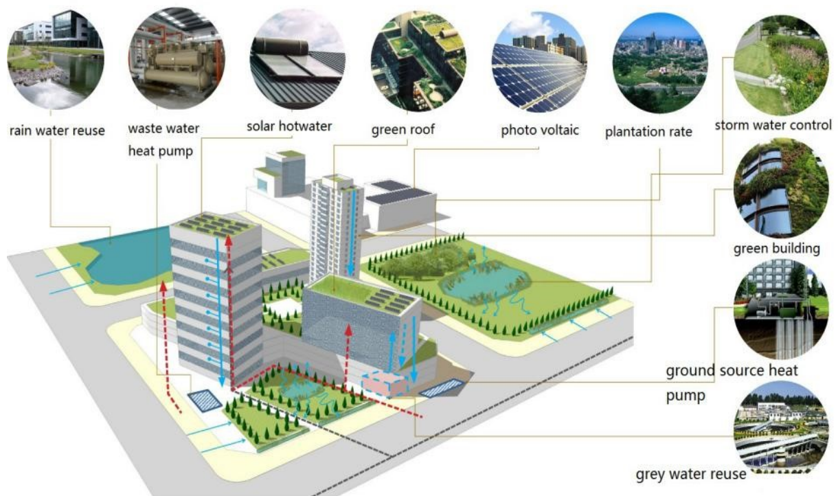
Fig.5. Technical routes in Shougang positive climate project
