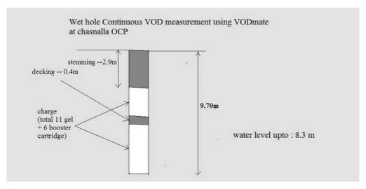
Fig. 9. Wet hole VOD Measurement using VODmate at Chasnalla OCP
