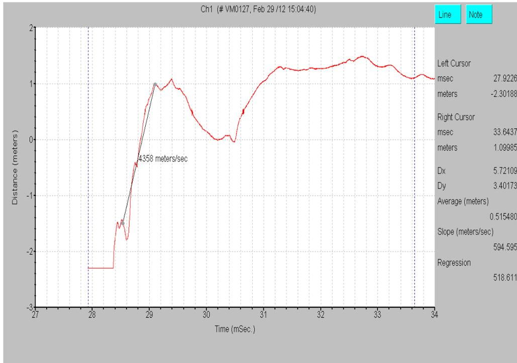
Fig. 7. Analysis on Blastware for Jamunia Mines
