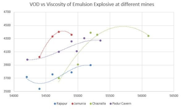
Figure 14: VOD of Emulsion Explosive Plotted Against Viscosity for 4 DifferentMines/Geology
