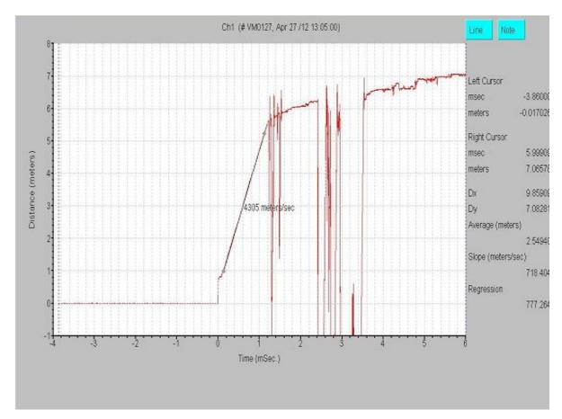
Fig. 12. VOD Analysis on Blastware for Padur Project
