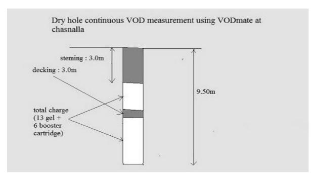
Fig. 10. Dry hole VOD Measurement Using VODmate at Chasnalla OCP
