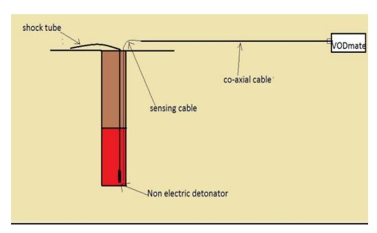
Fig. 2. VODmate Setup in a Single Hole Kept for the Continuous Monitoring
