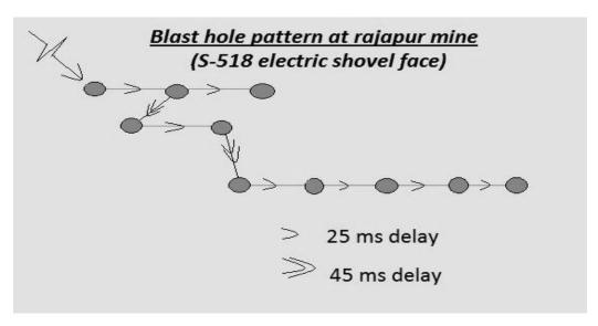
Fig. 4. Blast Design at Rajapur Mines
