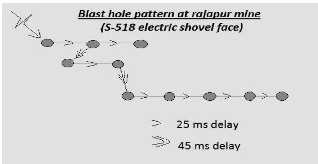
Fig. 4. Blast Design at Rajapur Mines
