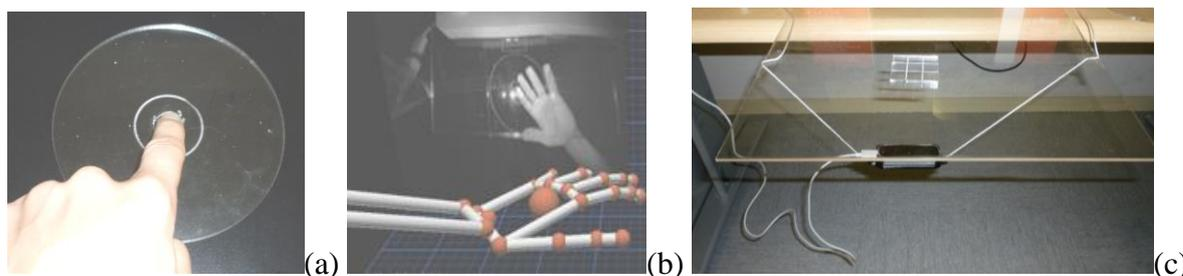
**Figure 1: (a) Plexiglas CD (b) Detection across the support (c) Leap is suspended under the Plexiglas support**
