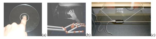
Figure 1: (a) Plexiglas CD (b) Detection across the support (c) Leap is suspended under the Plexiglas support
