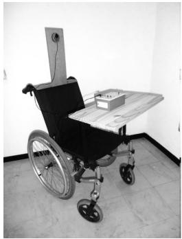
Fig. 1. Speech synthesis commanded by movements of head.
