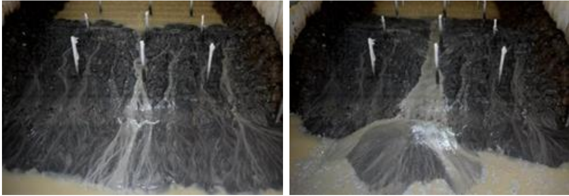
Fig .4. Tailing dam break breach evolution
