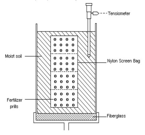
Fig. 1. Schematic diagram of the system used for measuring potassium nitrate and urea release in sandy soil.
