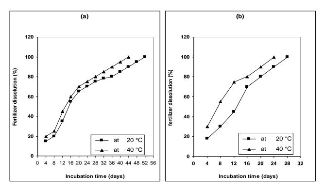
Fig. 5. Effect of temperature on dissolution for potassium nitrate and urea fertilizer having the same treatment  $Ex_3$ .
