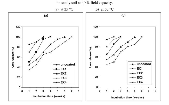
Fig. 9. Releasing rate of uncoated and coated urea in sandy soil at 40 % field capacity.
