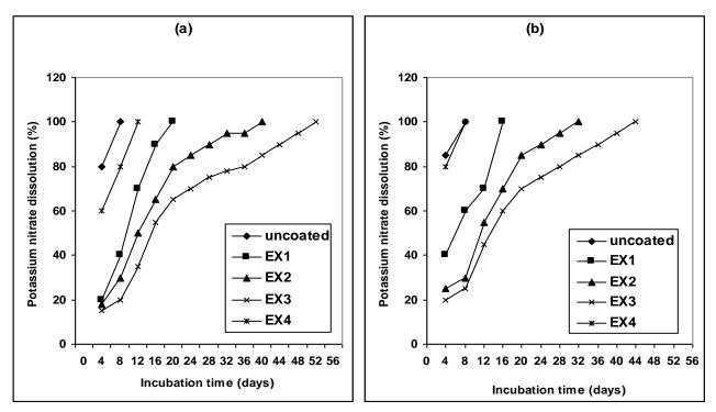
Fig. 2. Dissolution rate of uncoated and coated potassium nitrate in water. a) at 20 °C b) at 40 °C
