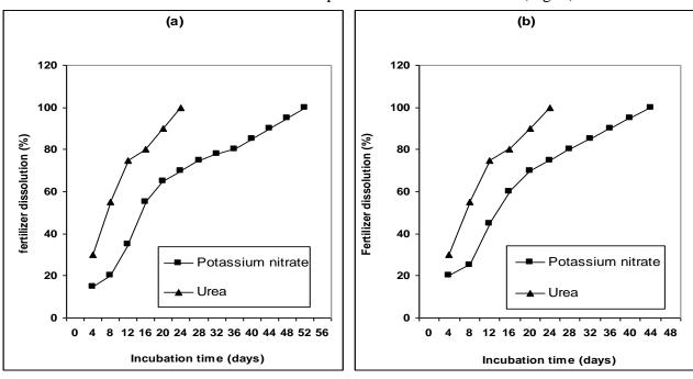
Fig. 4. Comparison between dissolution rates of potassium nitrate and urea fertilizers having the same treatment Ex<sub>3</sub>.a) at 20 °Cb) at 40 °C
