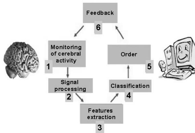
Figure 1: Six steps involved in BCI performing (source [12]).
