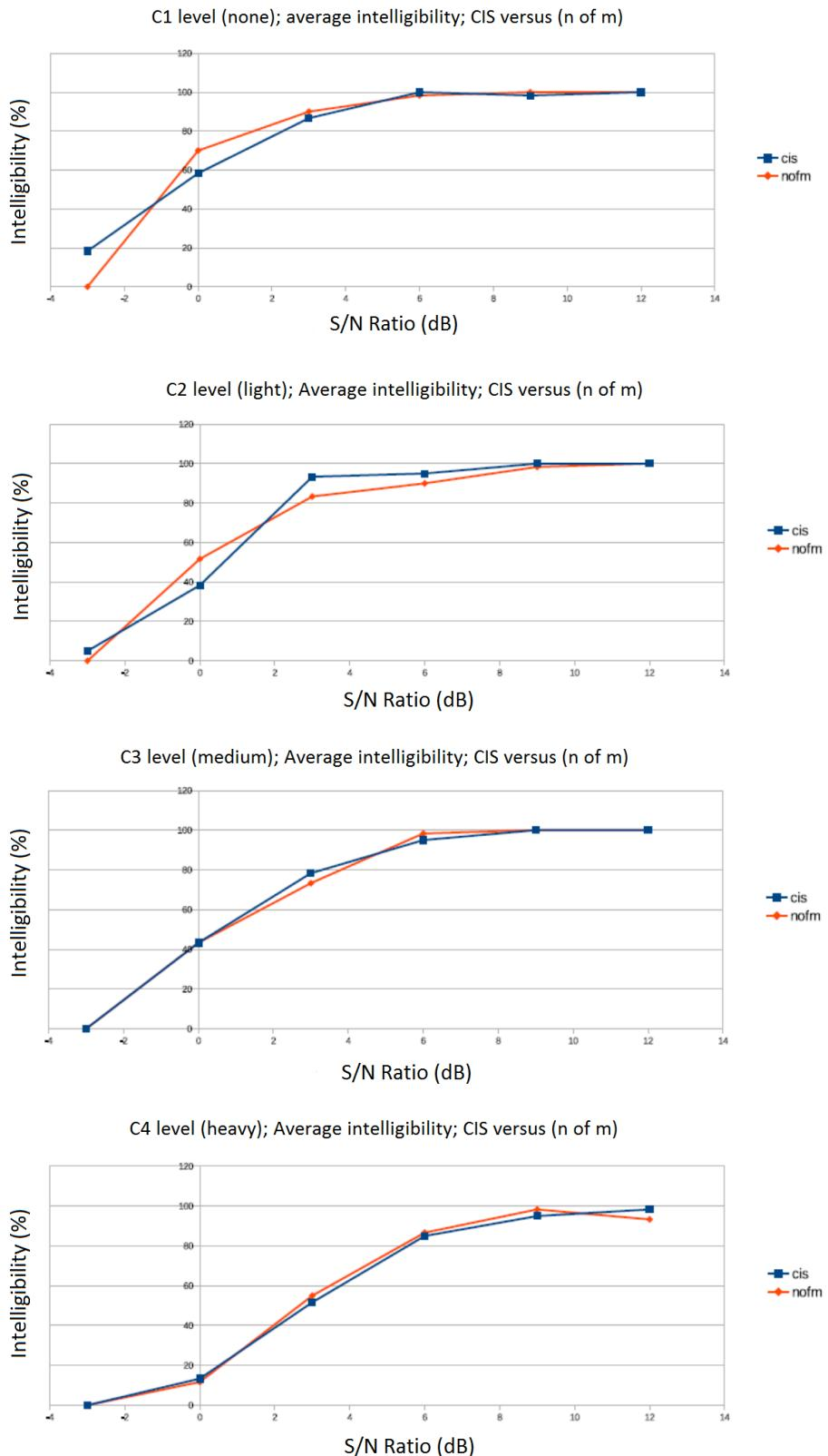
Fig. 4. Recognition percentages according to the microphone encrusting level (C1=none, C2=light, C3=medium, C4=heavy)
