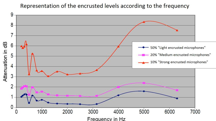
Fig. 3. Representation of the microphones « encrusting » according to the frequency, given in percentiles
