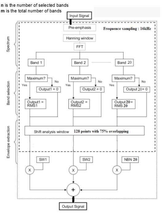
Fig. 2. Representation of cochlear implant coding
