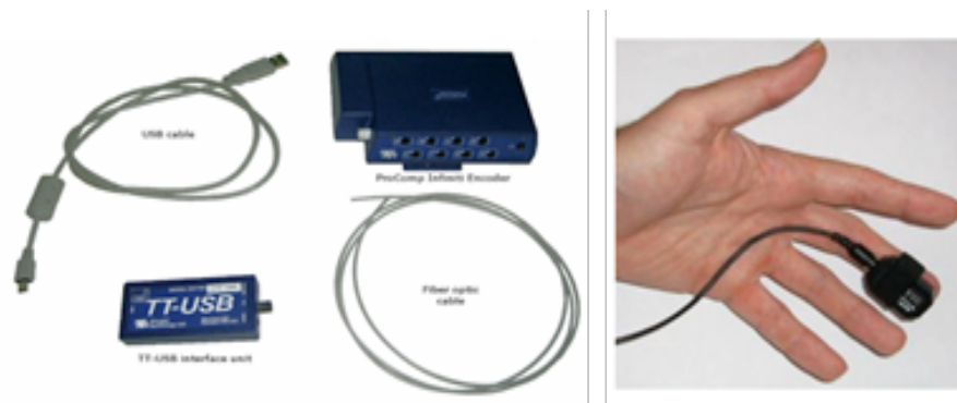
Fig. 2. The Procomp infinity encoder and the blood volume pulse sensor.
