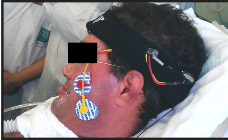
Fig. 6. Subject suffering of ALS; he controls with a sensor EMG (jaw) a demonstrator AAC generated with EDiTH2.
