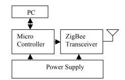
Fig.2 The system architecture at the doctor end
