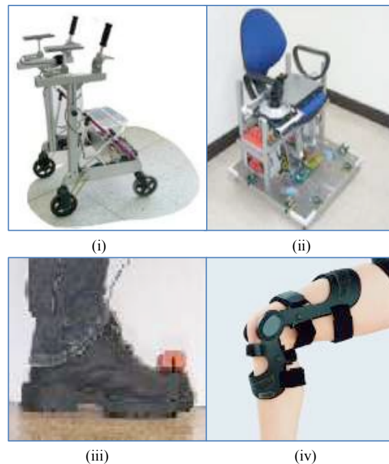
Fig. 3. Mobility Assistive Devices: (i) Simbiosis Walker [10] ; (ii) Robotic Wheelchair [11]; (iii) Shoe-mounted inertial navigation system [12]; (iv) Knee Orthosis [13]
