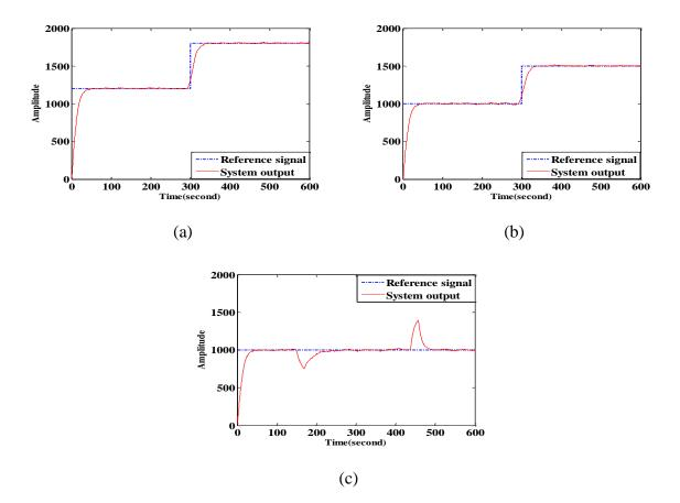
Fig 3: Reference with respect to response of DC motor experimental setup employed  $L_1$  adaptive controller for (a) Input 1, (b) Input 2, (c) Input 3.
