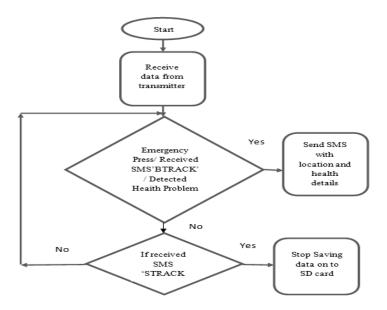
Fig.6. Flow chart Receiver Section
