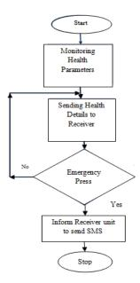
Fig.5. Flow chart of Transmitter Section
