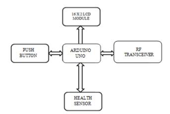
Fig.1. Block diagram of transmitter section
