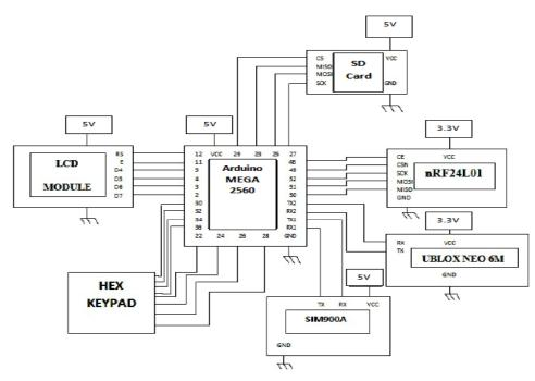
Fig.4. Circuit diagram of receiver section
