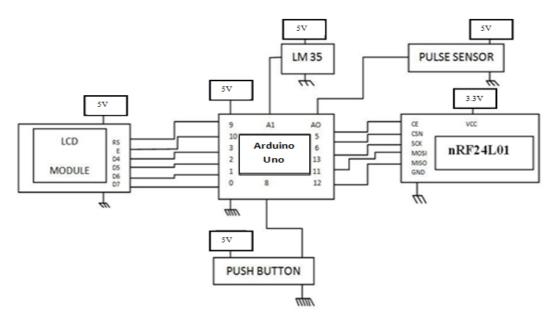
Fig.3. Circuit diagram of transmitter section
