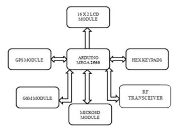
Fig.2. Block diagram of receiver section
