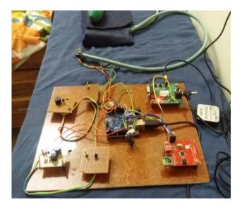
Figure 6. Experimental set up for REMP using Arduino and Zigbee
