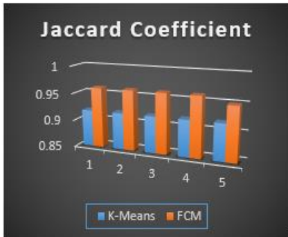
Figure 8. Jaccard Coeff of 5 variant kidney MRI images applying K-Means and FCM methods
