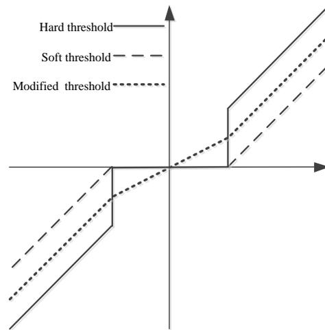
Fig.12. Schematic Diagram of the Improved Threshold Function
