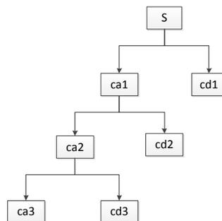
Fig.11. The Structure of Three Layer Wavelet Decomposition
