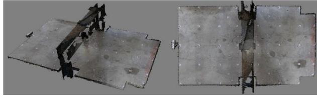
Fig.2. Three Dimensional Point Cloud Reconstruction Effect of Box Girder Specimen
