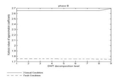
Fig.2. Kurtosis Values of Approximate Coefficients for Phase B Current Plotted with Respect to DWT Decomposition Level
