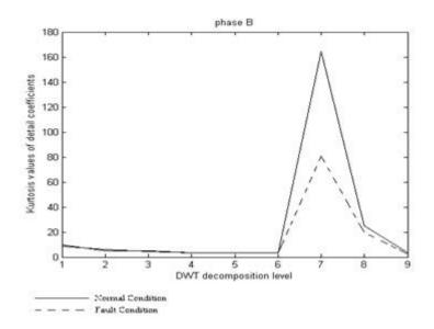
Fig.4. Kurtosis Values of Detail Coefficients for Phase B Current Plotted with Respect to DWT Decomposition Level
