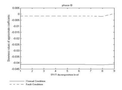
Fig.6. Skewness Values of Approximate Coefficients for Phase B Current Plotted with Respect to DWT Decomposition Level
