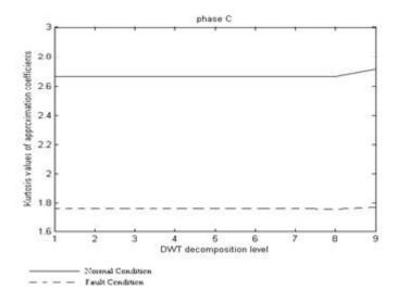
Fig.3. Kurtosis Values of Approximate Coefficients for Phase C Current Plotted with Respect to DWT Decomposition Level
