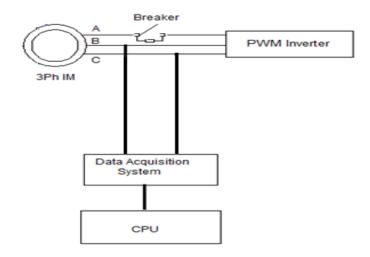
Fig.1. Experimental Model for Assessment of Single Phasing of a PWM Fed Induction Motor
