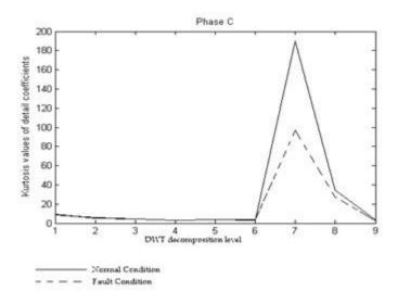
Fig.5. Kurtosis Values of Detail Coefficients for Phase C Current Plotted with Respect to DWT Decomposition Level
