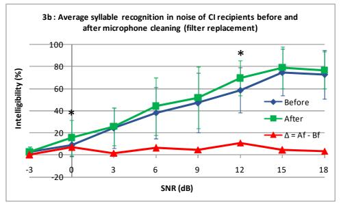
Figure 3: Recognition percentages before and after cleaning the microphone according to the cleaning procedure, "brush and blow" (3a) and filter replacement (3b). The cleaning effect  $\Delta$  is also represented.
