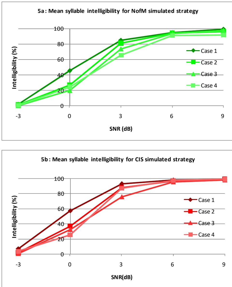
**Figure 5: Effect of the microphone loss of sensitivity on the recognition of the syllables, according to the microphone loss of sensitivity, for the NofM and the CIS strategies.**
