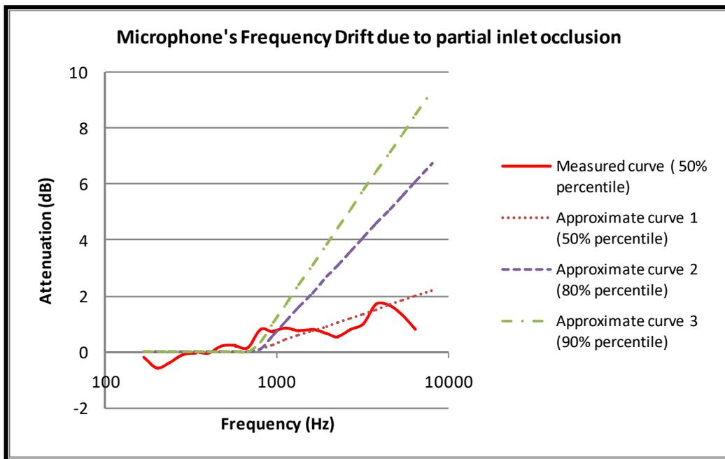
Figure 3 : Simulation of the microphone loss of sensitivity.
