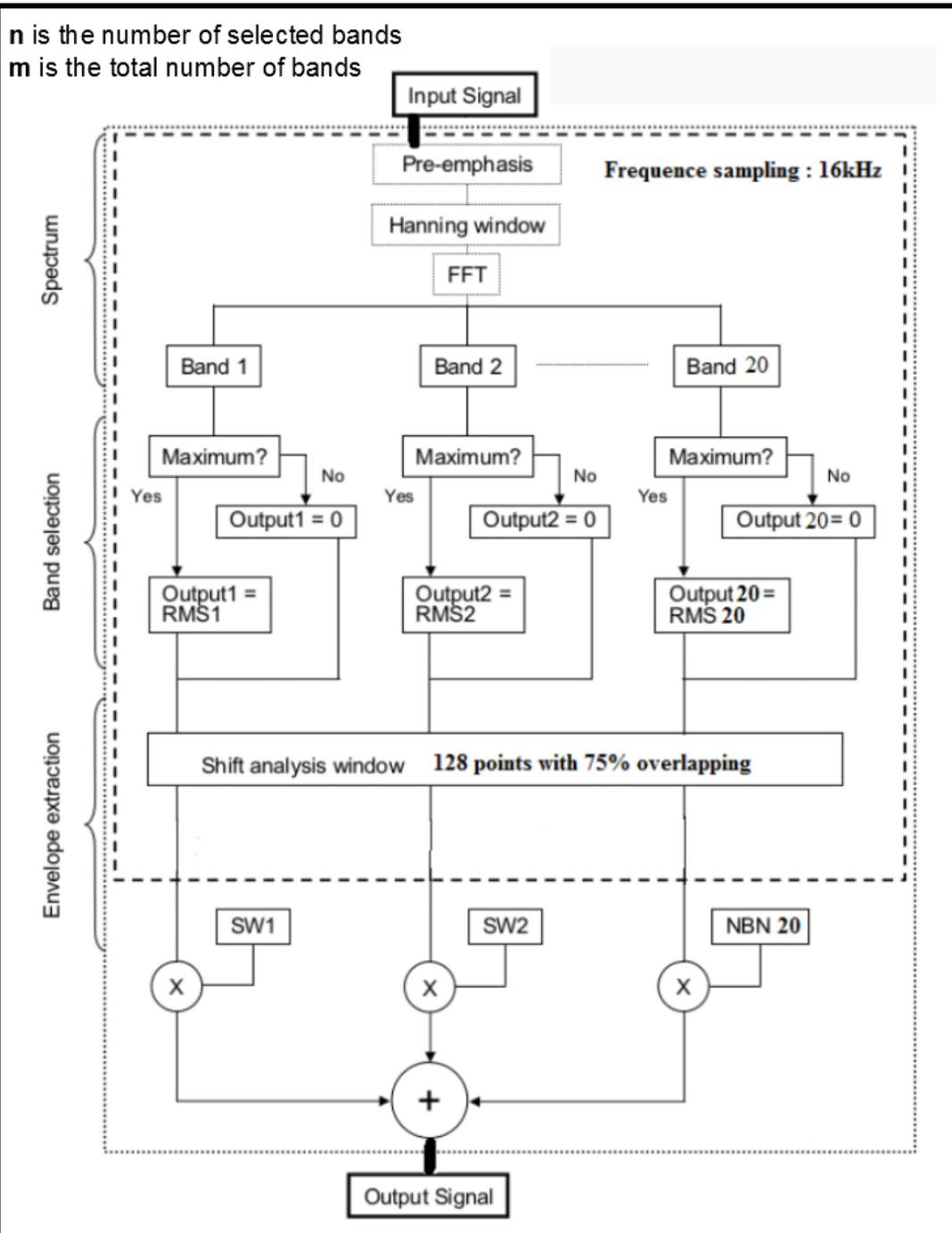
Figure 1: Simulation of cochlear implant coding by a vocoder.
