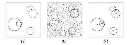
Fig. 2. The experiment on the synthetic images (I): (a) The original image, (b) The image with 1618 noises, (c) The detected circles with the proposed algorithm
