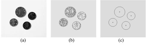
Fig. 5. The experiment on the real image (II): (a) The original image, (b) The edge image, (c) The detected circles with the proposed algorithm
