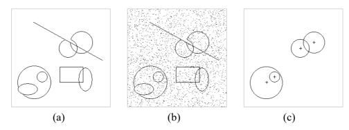
Fig. 3. The experiment on the synthetic images (II): (a) The original image, (b) The image with 2340 noises, (c) The detected circles with the proposed algorithm
