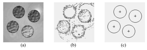
Fig. 4. The experiment on the real image (I): (a) The original image, (b) The edge image, (c) The detected circles with the proposed algorithm
