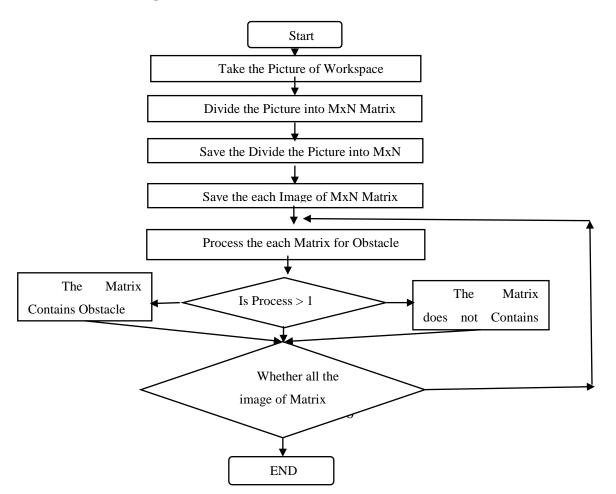
**Design Flow Chart for Automatic Obstacle Detection**
