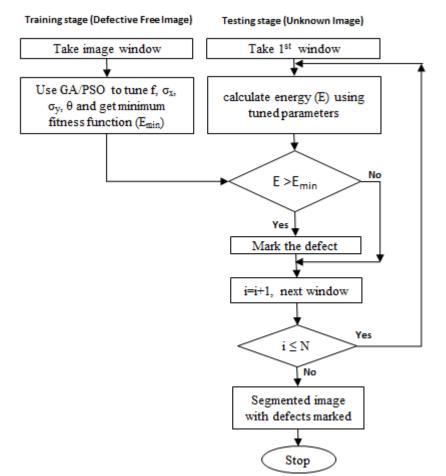
Fig. 2. Flow chart for training and testing stage of defect detection mechanism (N=total number of windows)
