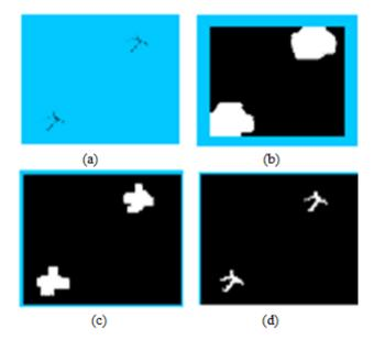
Fig. 5. Color Gabor filter results (a) Defected input color image with two cracks (b) Output image for window size 60X60 (c) Output image for window size 15X15 (d) Output image for window size 5X5
