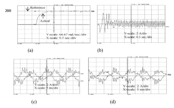
Fig.13. Experimental starting responses of the proposed fuzzy based CSI fed Synchronous Motor (CSIFSM). (a) Speed. (b) Stator current *i*a. (c) Steady-state currents *i*a and *i*b. (d) Steady-state currents *i*a and *i*c.
