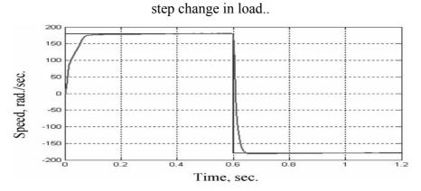
Fig.12. Simulated speed response of the proposed fuzzy based CSI fed Synchronous Motor (CSIFSM) drive for speed reversal of command speed.
