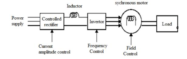
Fig.1 Drive configuration for open-loop CSI fed Synchronous Motor (CSIFSM) control The transformed version of equation 3 and 4 are:
