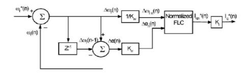
Fig.8. Fuzzy speed controller Construction
