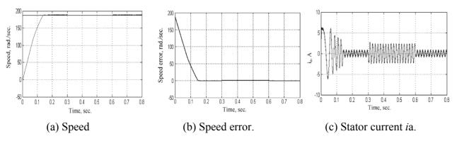
Fig.11. Simulation responses of the fuzzy based CSI fed Synchronous Motor (CSIFSM) drive for a
