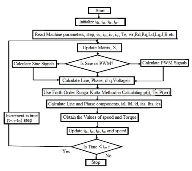
Fig.9 Flow charts for calculating steady state stability analysis (SSSA)
