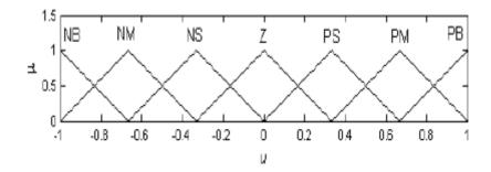
Fig.6. Membership functions for input e, de and u
