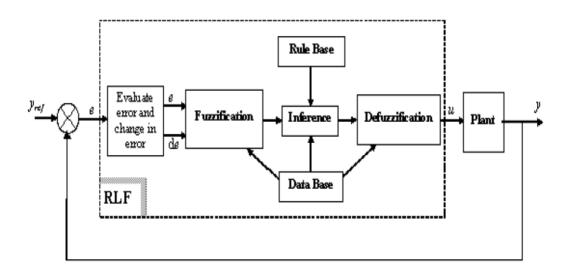
Fig.5 Basic structure of fuzzy control system
