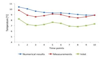
**Figure 4.** Comparison between numerical and real temperatures on the outlet face of exchanger B2 in the time
