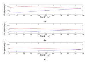
**Figure 7.** Temperature profiles in the downward (blue) and upward (red) pipe for exchanger B1 in I1
