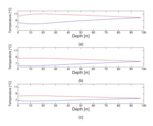
**Figure 8.** Temperature profiles in the downward (blue) and upward (red) pipe for exchanger B1 in I2
