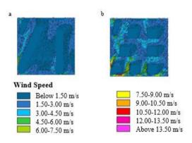
**Figure 6.** Wind Speed [m/s] - Scenarios Comparison at 13:00, h=1.5 m: a) BaseS, b) TowerS
