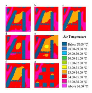
**Figure 5.** Air Temperature [°C] - Scenarios Comparison at 13:00, h=1.5m: a) BaseS, b) GRoofS, c) GWallS, d) Green S, e) BlueWS, f) WhiteBS, g) TowerS
