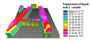
Figure 2. Temperature of facades and roofs at node 1 in ENVI-met for the Base Scenario at 13:00
