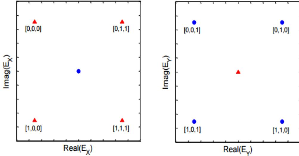
Fig 3. Constellation diagrams of PS-QPSK Signal (linearly polarized).
