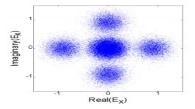
Fig.4. Constellation diagram of a PS-QPSK with the CMA equalizer (single polarization output)
