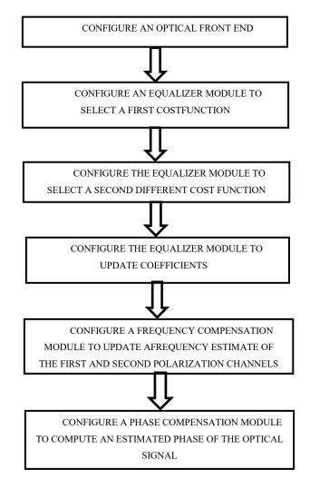
Fig. 1. Steps to form an optical PS-QPSK optical receiver
