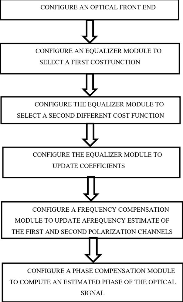
Fig. 1. Steps to form an optical PS-QPSK optical receiver
