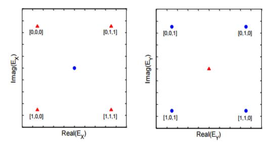
Fig 3. Constellation diagrams of PS-QPSK Signal (linearly polarized).
