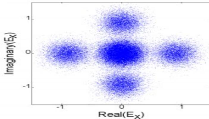
Fig.4. Constellation diagram of a PS-QPSK with the CMA equalizer (single polarization output)
