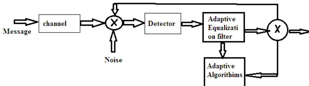
Fig.2. Adaptive Equalization
