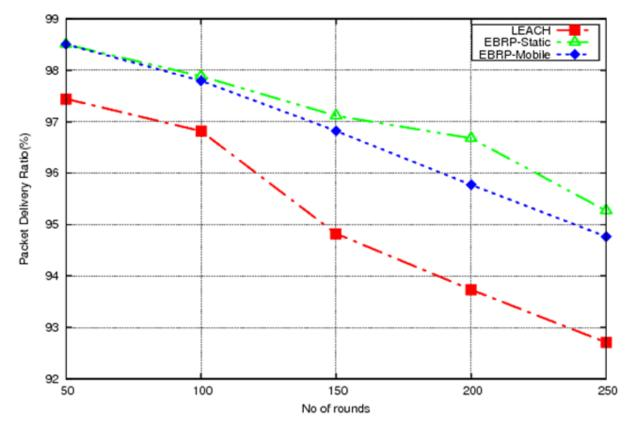
Fig.5 Number of rounds Vs Packet delivery ratio
