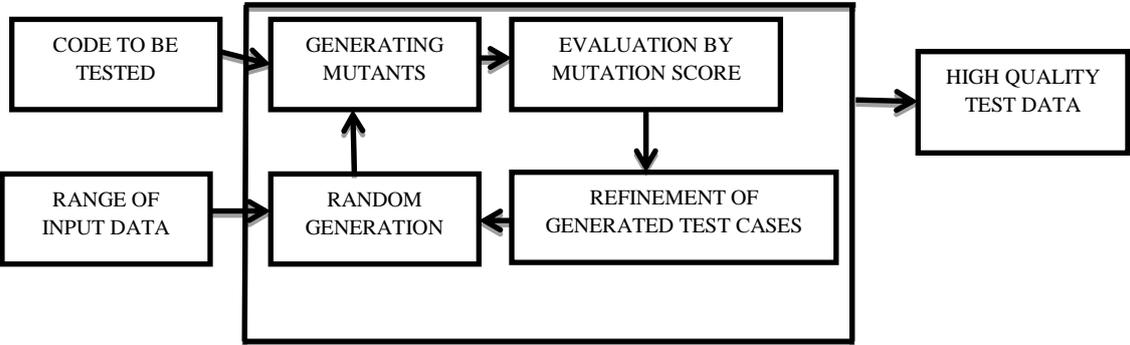
**Figure 5: Hirohide Haga et al [5] test case generation using Mutation Analysis and GA Algorithm**
