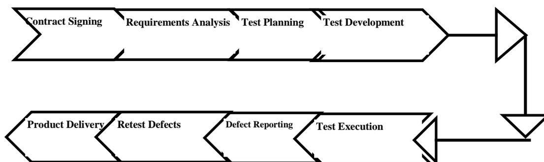
**Figure 1: Software Testing Life Cycle Process**
