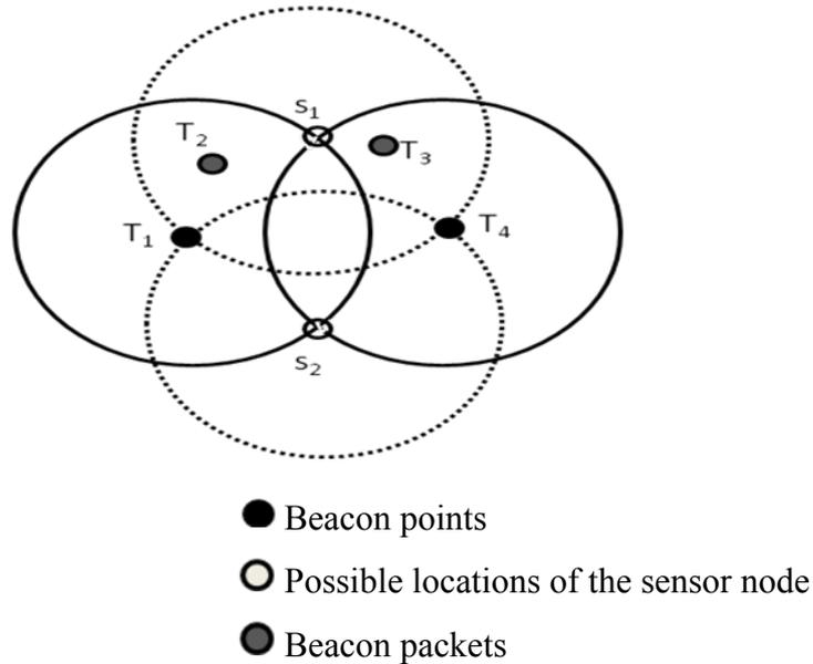
Fig.1. Possible locations of the sensor node.
