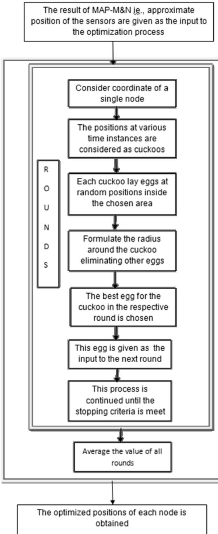
Fig.4. Localization steps used in MAP-M&N with CS-MAP algorithm
