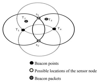
Fig.1. Possible locations of the sensor node.
