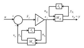
Figure 4. Block diagram representation with uncertain parameters
