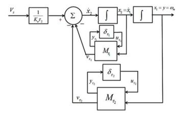
Figure 7. Block diagram of BLDC motor with uncertain parameters
