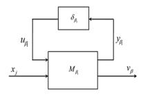
**Figure 3.** Representation of uncertain parameter  $\delta_{\beta_i}$  in upper LFT framework
