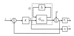
Figure 10. Closed loop structure of BLDC motor
