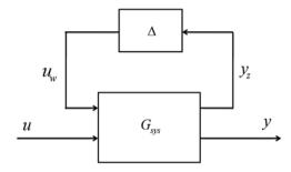
Figure 5. Upper LFT representation of the linear dynamical system
