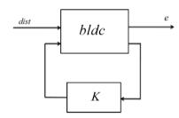
Figure 11. Close loop BLDC motor with  $H_{\infty}$  controller
