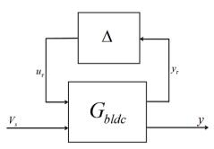
Figure 8. Upper LFT representation of BLDC motor
