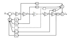
Figure 1. Block diagram representation of n<sup>th</sup> order linear dynamical system
