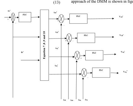
Figure 4. Block diagram of the fuzzy logic PI controller for DFOC approach of the DSIM
