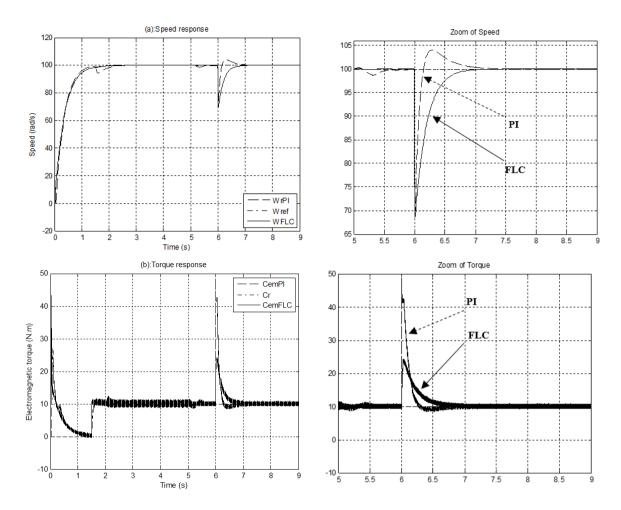
Figure 8. Speed and torque characteristic of an (DFOC) with PI and FLC controllers, at parametric variations (rotor resistance  $(R_{rl}=1.5*R_r)$ , moment of inertia  $(J_1=1.5*J)$ ).
