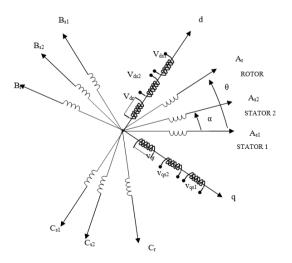
Figure 1. Doubly stator winding representation
