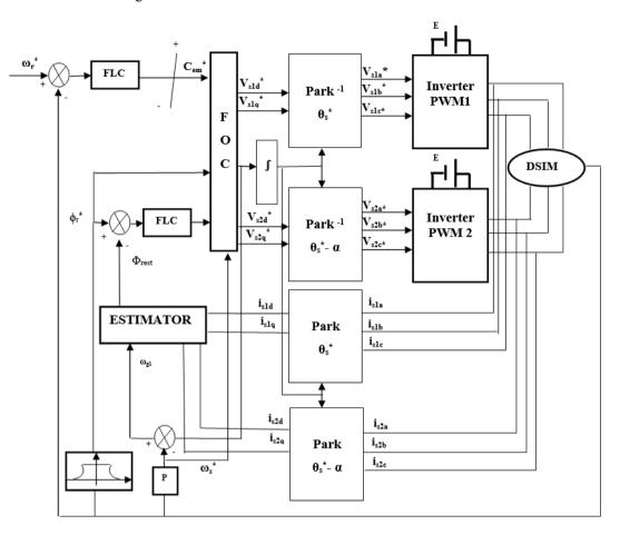
Figure 5. Structure of speed ordering for the DSIM
