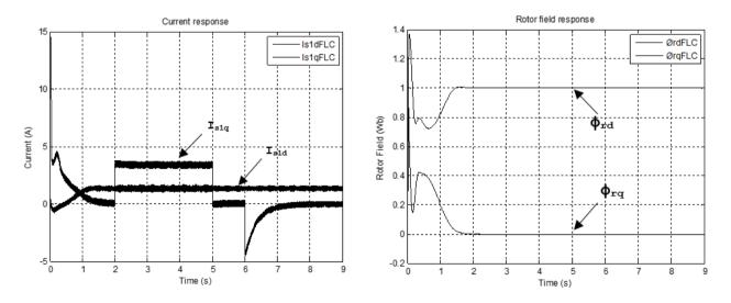
Figure 7. Decoupling and rotor field orientation
