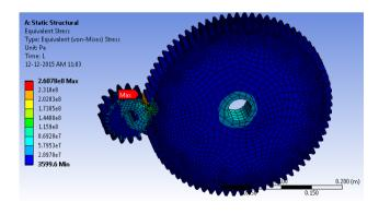
Figure 3. Bending stress distribution for steel C45 made gear pair
