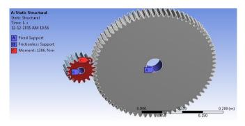
Figure 2. Boundary conditions for present analysis on spur gear pair
