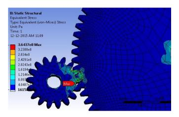
Figure 4. Bending stress distribution for HDPE made gear pair
