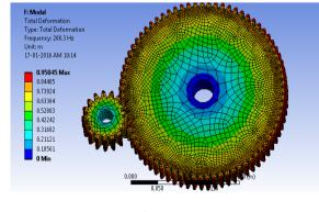
Figure 5. Modal displacement for C45 steel made gear pair
